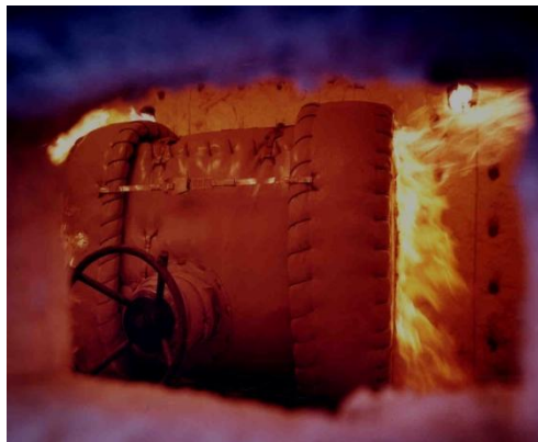
FIG. 4 – Darmatt Furnace test for Hydrocarbon Pool Fire
