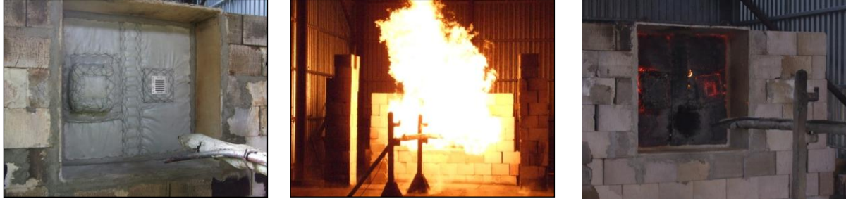
FIG. 3 – Before, during, and after a 180 minute Jet Fire Test – Flat Panel protected with Darmatt Jet Fire jackets - with corner and edge features, lacing and Darvent
