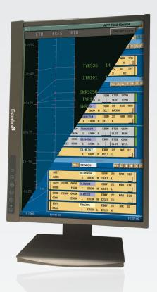
Air Traffic Controllers are using more and more tools to display an ever-increasing load of information. That is why more and more visualization capabilities with respect to display size and resolution are needed. The CODIS® 24" ADP-361 auxiliary display is especially designed to meet these concerns.
