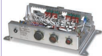
DC contactor with Hall Effect sensor for military and aircraft applications
