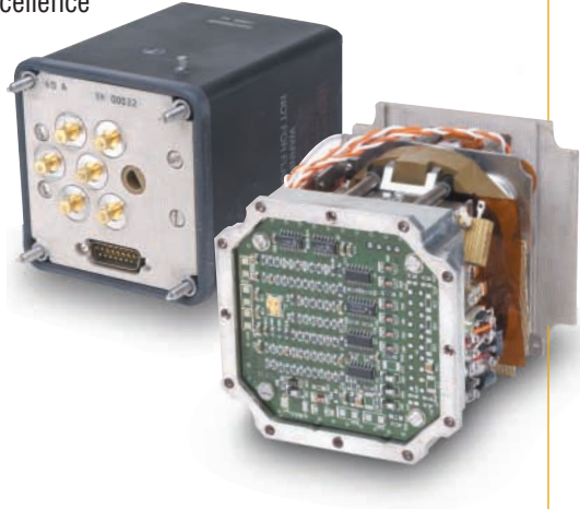
Electrical load control unit for commercial aircraft
