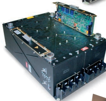
DC power distribution assembly for military transport aircraft
