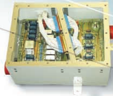
Wiring integrated assembly box for helicopter
